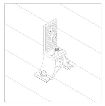
3. Fix the L foot connector to corrubracket to 16 N·m using a 13mm socket seat.
