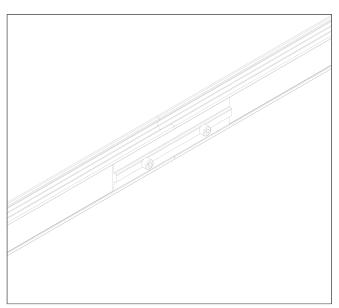
**5.** Connect multiple rails by using rail splice (if required per system design)
