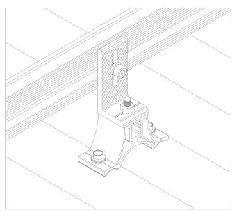
4. Connect rails to L foot connector to 16 N·m using a M6 Allen key or hex driver bit
